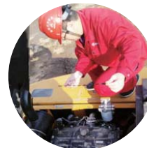
Inspect the situation of engine oil
