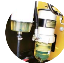
Water drain valve and check valve of fuel tank
